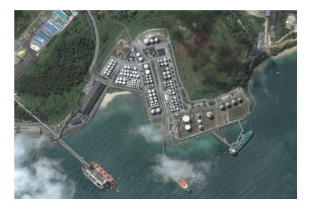
**The Liquid Bulk Terminal (TGL)** consists of a 220 meter-long quay and 12 meters (39.37 feet) deep with mooring on both sides (2 berths), through which the handling of the following products is made: Caustic soda, dichloroethane, EG, styrene, MTBE, benzene, etc..
