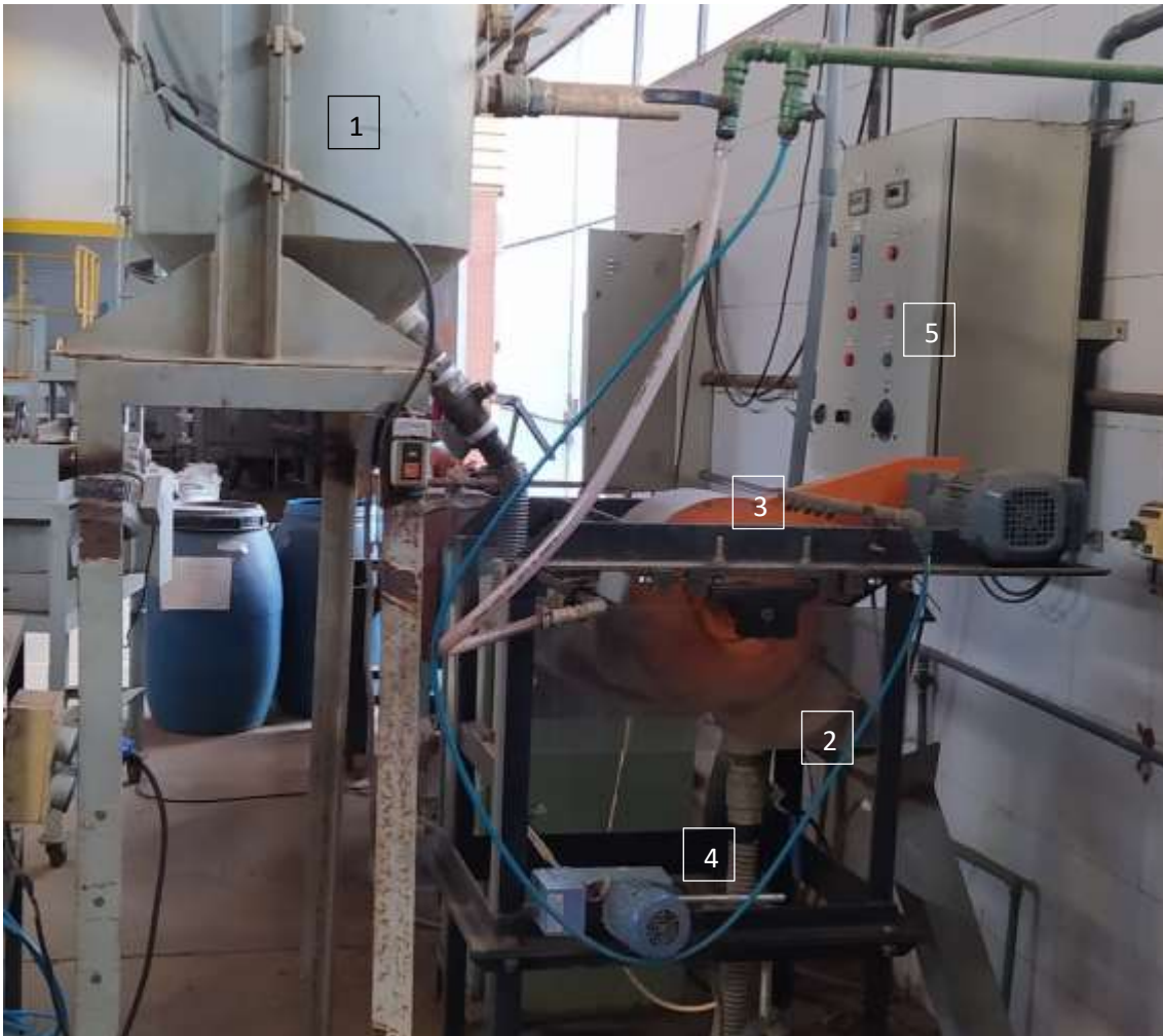
Figure 3: The WDL8 at the pilot-plant. 1- Feed bin, 2 – Separation chamber, (3) Drum, (4) Tailings valve/hose, (5) control panel.
