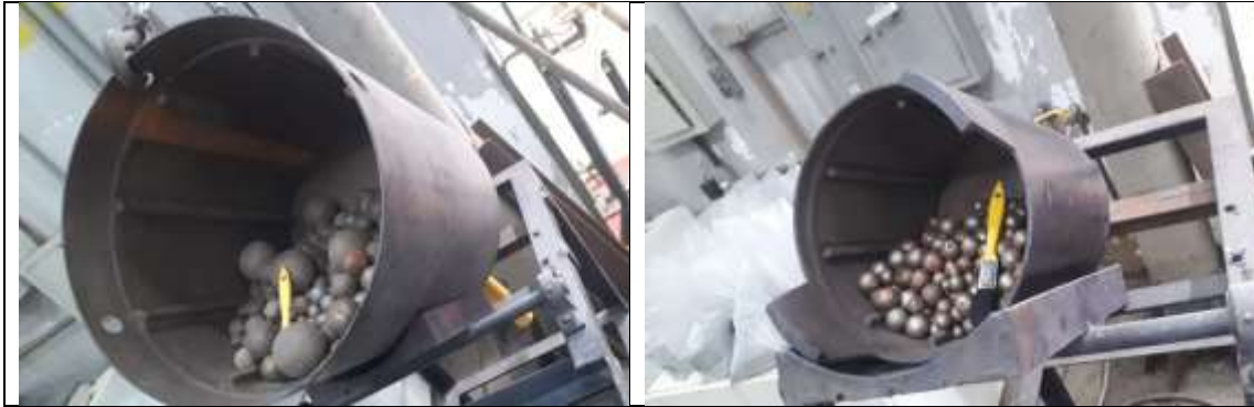
Figure 4: The 0.5x0.5 m batch ball mill with the 75 mm equilibrium ball charge (left) used in the primary grinding tests and the 250x250 mm batch ball mill with the 25 mm equilibrium ball charge (right) used in the magnetic concentrate pellet feed grinding tests.
